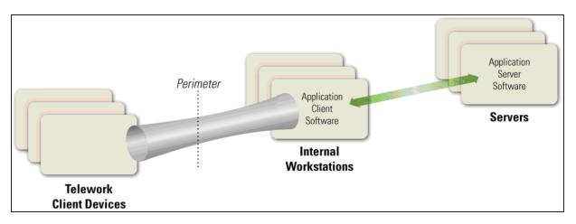
Figure 2-3. Remote Desktop Access Architecture
