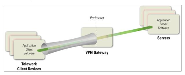
Figure 2-1. Tunneling Architecture
