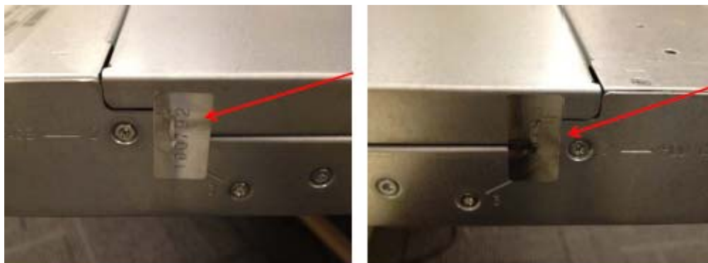
Figure 10 – Tamper-Evidence Labels on Side of ESKM
