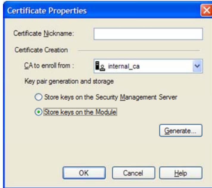
Figure 11 – Configuring the module to generate RSA keys with DKM on a per-certificate basis
