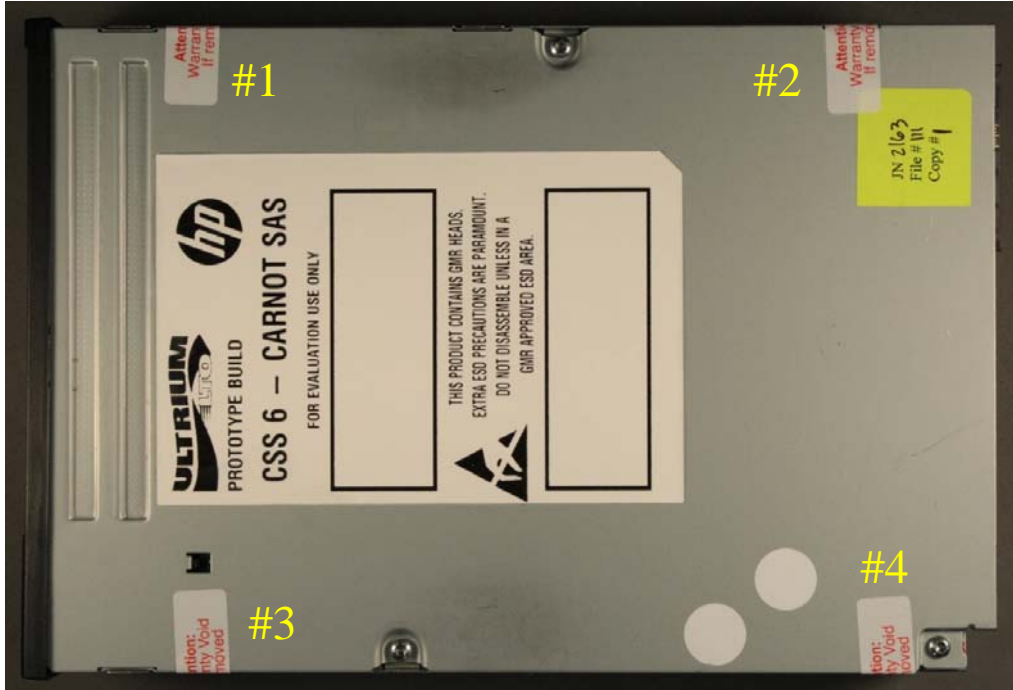
Figure 6 – Tamper Evident Seal Locations #1-4 Half-height Top
