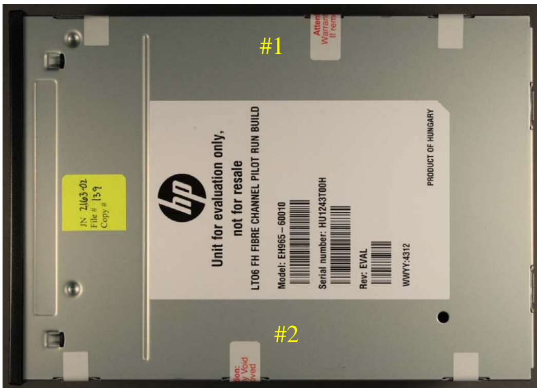
Figure 4 – Tamper Evident Seal Locations #1 & #2 Full-height Top
