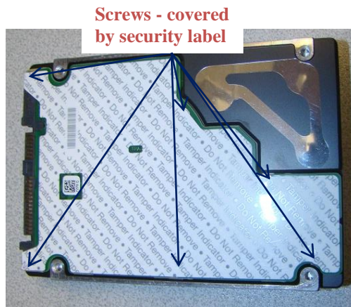
Figure 10: Enterprise Capacity® 3.5, HDD v4 (SAS/SATA) Screw covered by Security label
