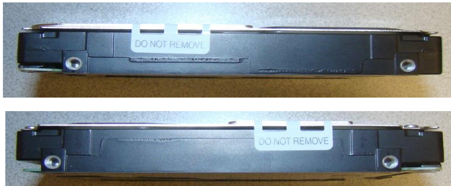
Figure 7: Enterprise Performance® HDD v5, Enterprise Performance® HDD v8, Enterprise Capacity® HDD v3 (SAS Interface) security labels on sides of drive
