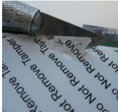
Figure 3: Tamper Evidence on Tamper Seal
