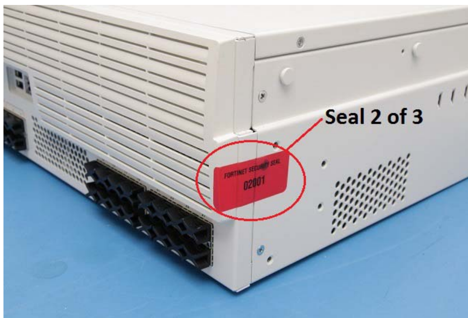
Figure 5: FortiGate-3600C Front Cover Plate Seal, right side
