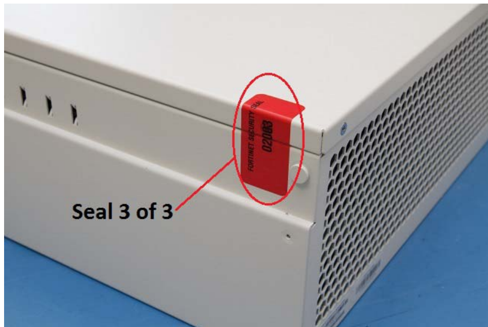
Figure 6: FortiGate-3600C External Enclosure Seal, top, right side
