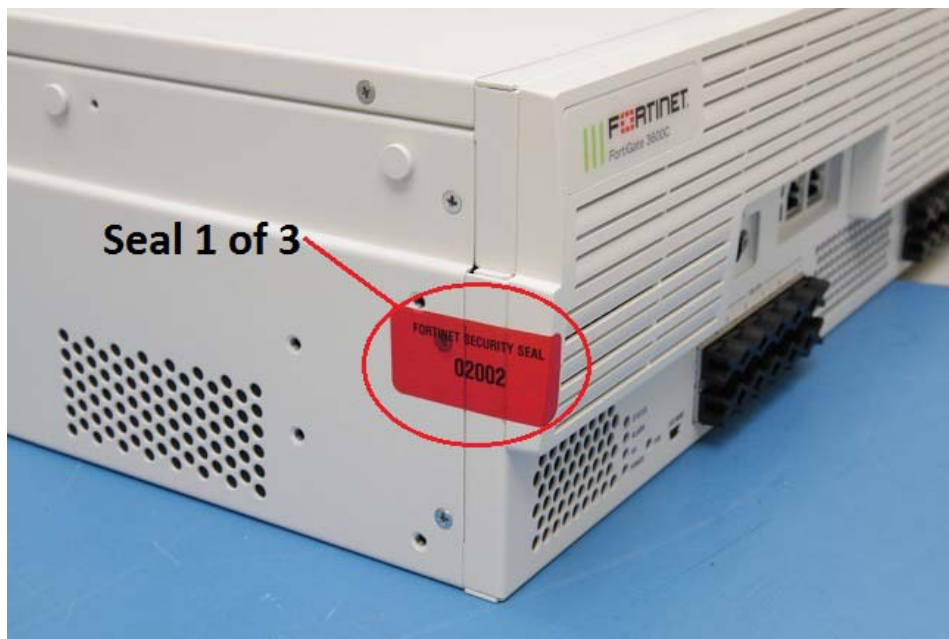
Figure 4: FortiGate-3600C Front Cover Plate Seal, left side
