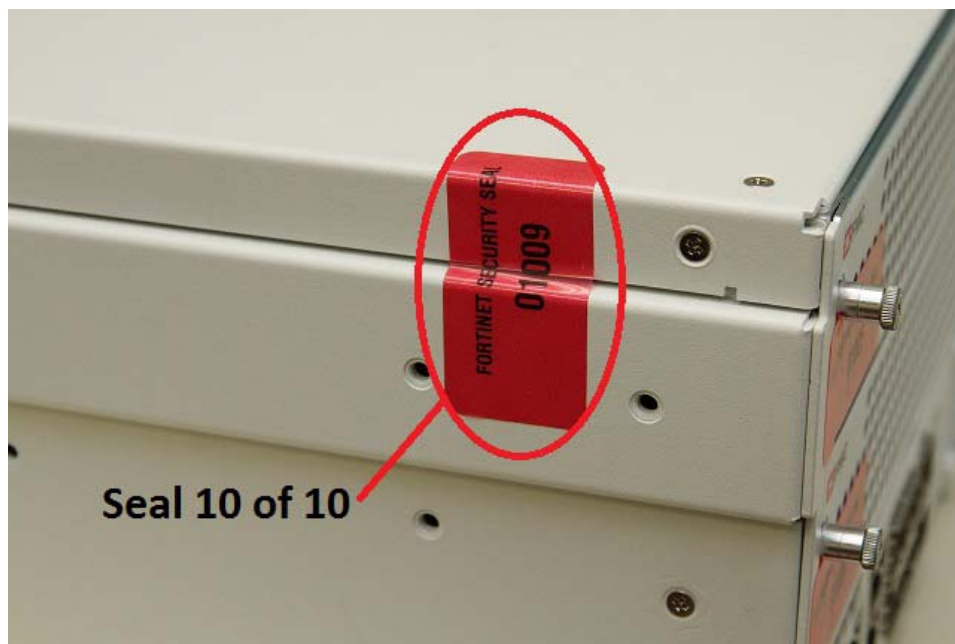
Figure 9: FortiGate-3950B External Enclosure Seal, top, left side
