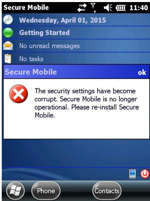
Figure 3 - Screenshot of corruption in Secure Mobile FIPS 140-2 Cryptographic Module
