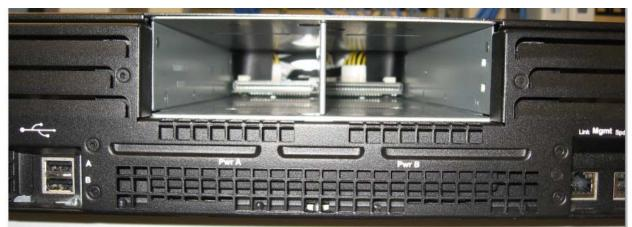
Figure 5 - Rear panel with Power supplies removed
