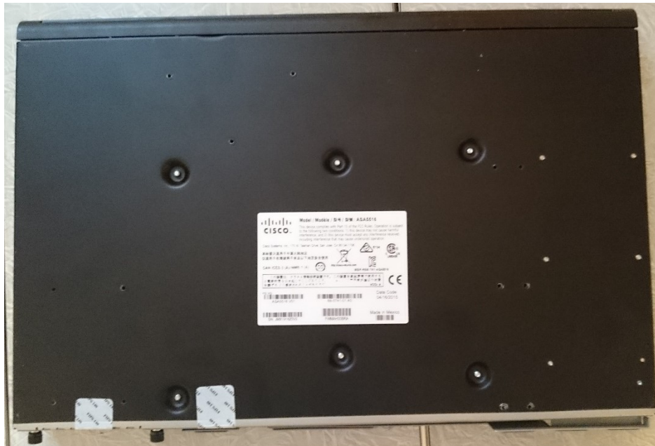
Figure 54 ASA 5516-X Bottom TEL Placement
