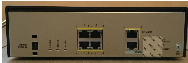
Figure 27 ASA 5506H-X Rear TEL Placement
