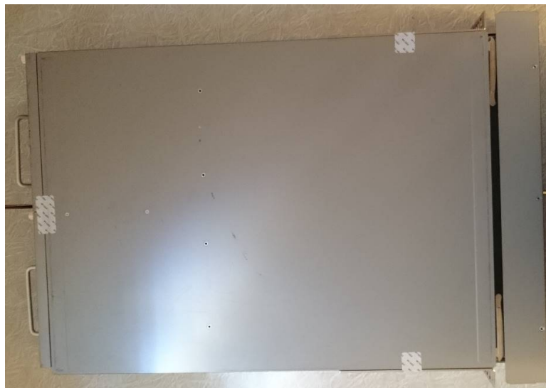
Figure 75 ASA 5585-X Bottom TEL Placement
