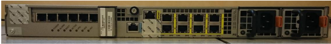
Figure 63 ASA 5545-X Rear TEL Placement
