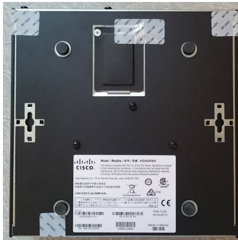
Figure 30 ASA 5506H-X Bottom TEL Placement
