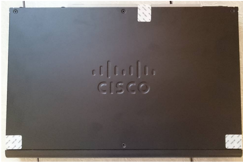
Figure 35 ASA 5508-X Top TEL Placement
