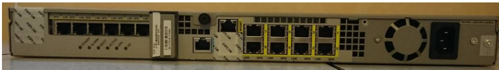
Figure 57 ASA 5525-X Rear TEL Placement
