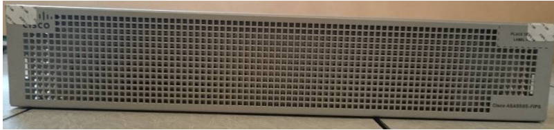
Figure 73 ASA 5585-X Opacity Shield and Front TEL Placement
