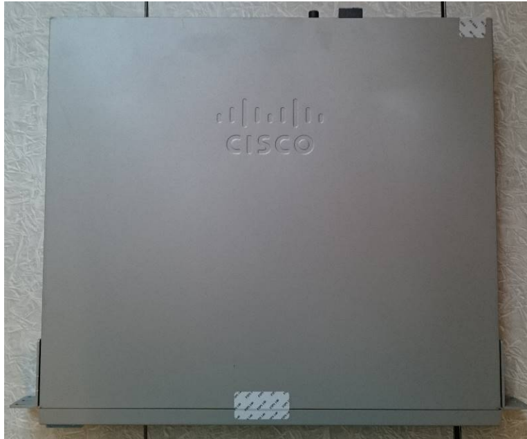
Figure 59 ASA 5525-X Top TEL Placement
