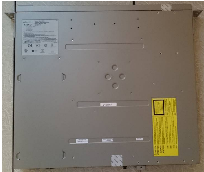
Figure 42 ASA 5512-X Bottom TEL Placement
