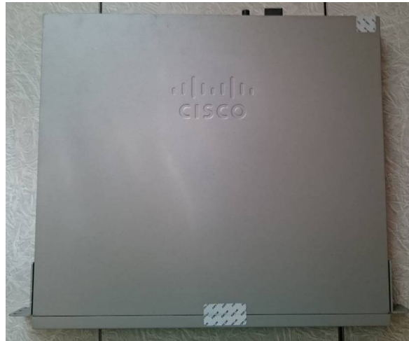
Figure 47 ASA 5515-X Top TEL Placement
