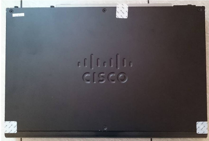
Figure 53 ASA 5516-X Top TEL Placement
