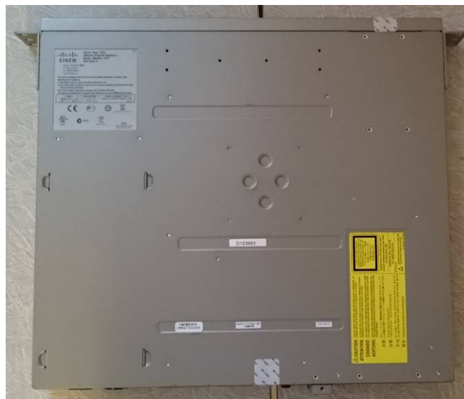
Figure 60 ASA 5525-X Bottom TEL Placement
