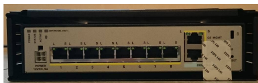
Figure 22 ASA 5506-X and ASA 5506W-X Rear TEL Placement
