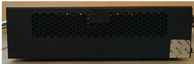
Figure 28 ASA 5506H-X Left Side TEL Placement
