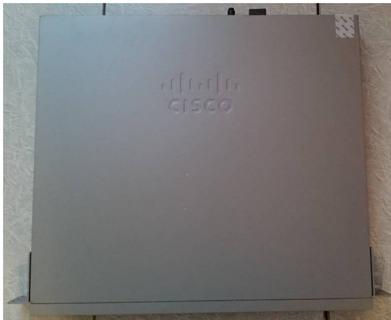
Figure 41 ASA 5512-X Top TEL Placement
