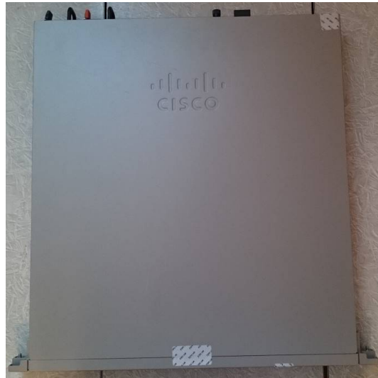
Figure 71 ASA 5555-X Top TEL Placement
