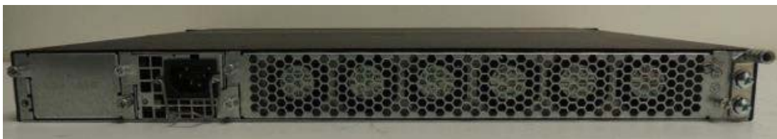
Figure 15 - BR-CES-2024F-4X-AC backside with Power supply: RPS9 (AC Power supply)
