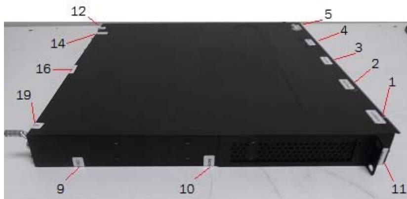
Figure 25 - Left side view of Brocade CER 2024F-4X-RT device with security seals
