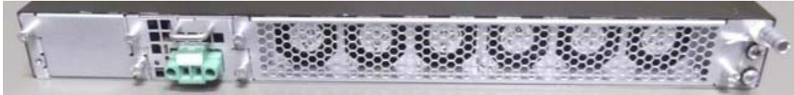
Figure 17 - BR-CES-2024F-4X-DC backside with Power supply: RPS9DC (DC Power supply)
