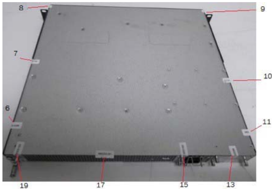
Figure 32 - Bottom view of Brocade CES 2024C-4X device with security seals
