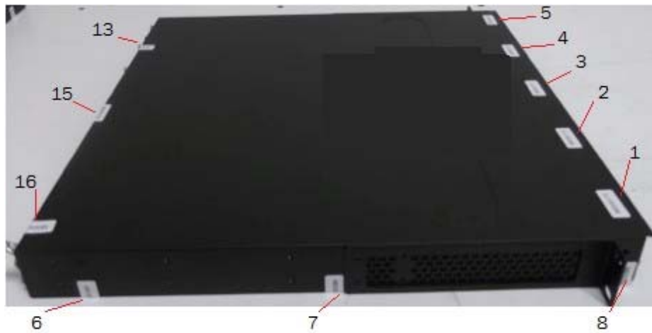
Figure 20 - Left side view of Brocade CER 2024C-4X-RT device with security seals
