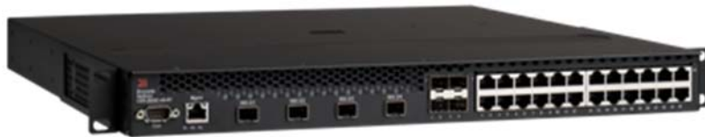
Figure 4 - BR-CER-2024C-4X-RT-DC with Base: BR-CER-2024C-4X-RT-DC and License: SW-CER-2024-RTUPG
