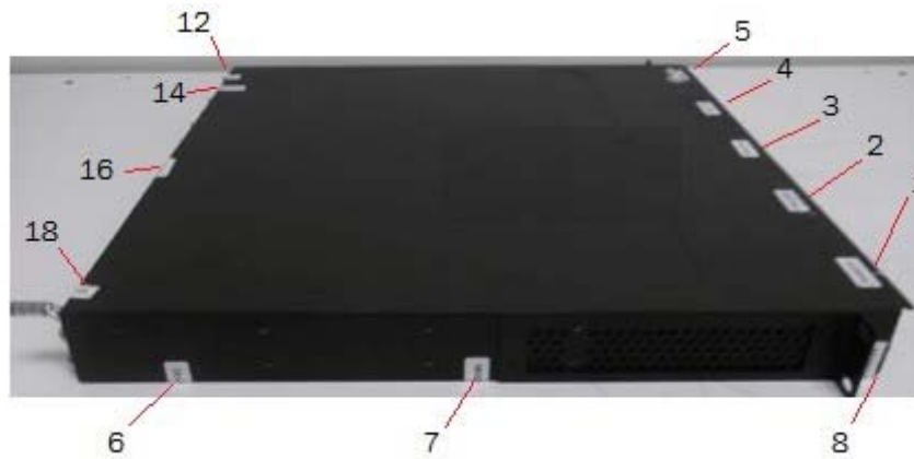
Figure 30 - Left side view of Brocade CES 2024C-4X device with security seals
