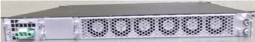
Figure 3 - BR-CER-2024F-4X-RT-DC backside with Power supply RPS9DC (DC Power Supply)
