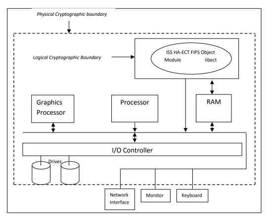
Figure 1 – Physical/Logical Cryptographic Boundary
