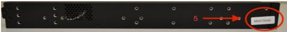
Figure 110 - ICX7250 48 ports left side seal location (tamper label #5)
