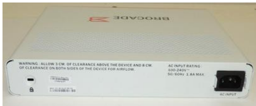
Figure 20 - Back side with power supply
