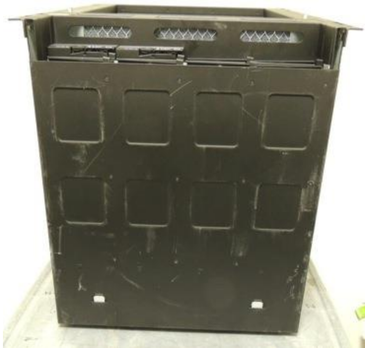
Figure 79 - Bottom view of the Brocade SX1600
