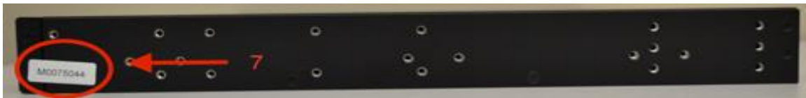
Figure 114 - ICX7250 48 ports right side seal location (tamper label #7)
