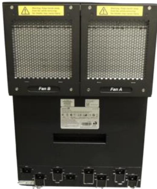
Figure 77 - Back side view of the Brocade SX1600 with fans and power supply
