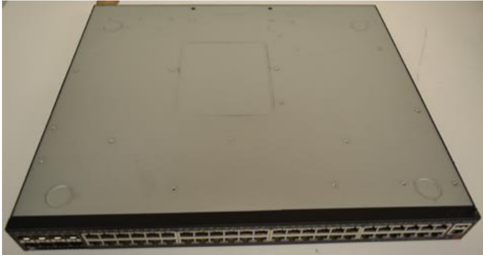
Figure 52 - Bottom side of the module ICX7250-48
