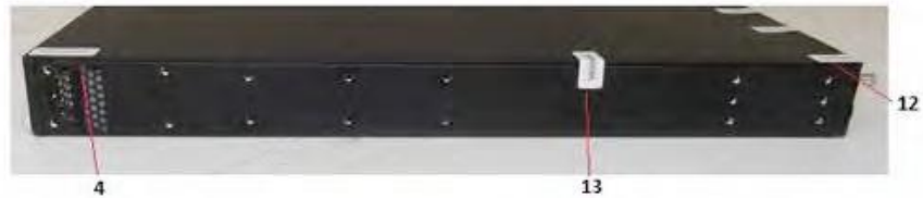
Figure 116 - ICX7750 - Right and top side view with tamper evident label security seals
