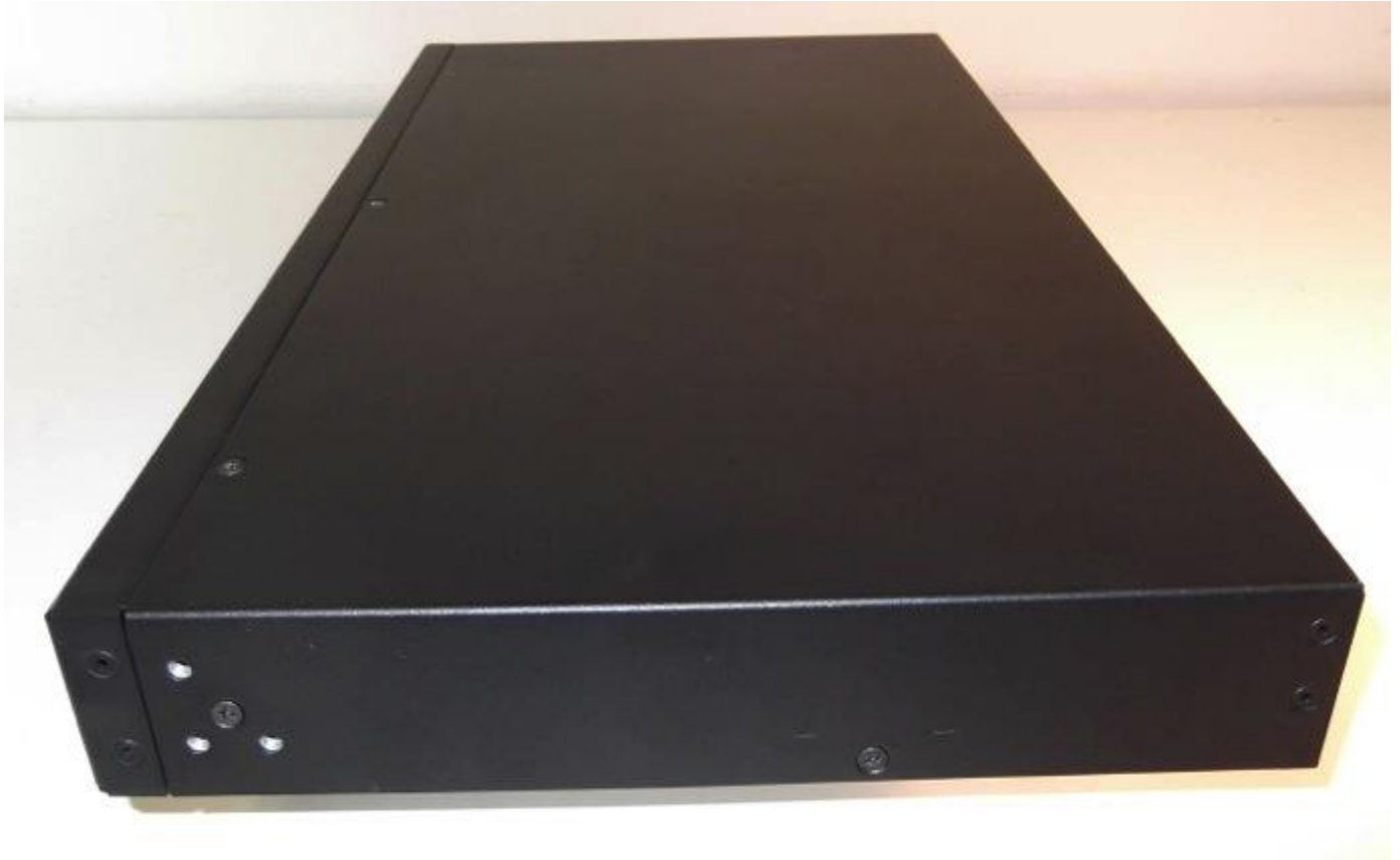
Figure 10 - Right side of the ICX 6450-24P (equivalent to the ICX 6450-24 configuration)
