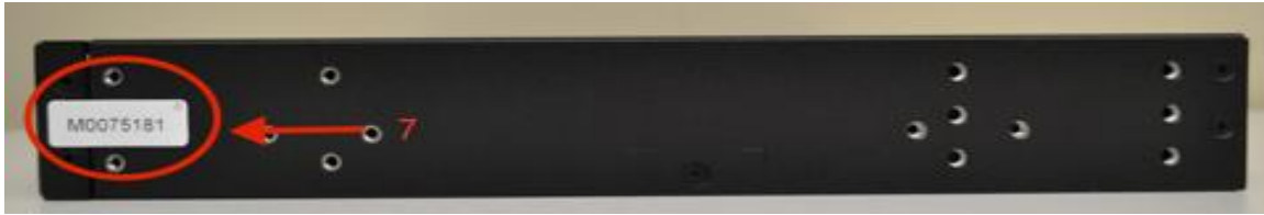
Figure 113 - ICX7250 24 ports right side seal location (tamper label #7)
