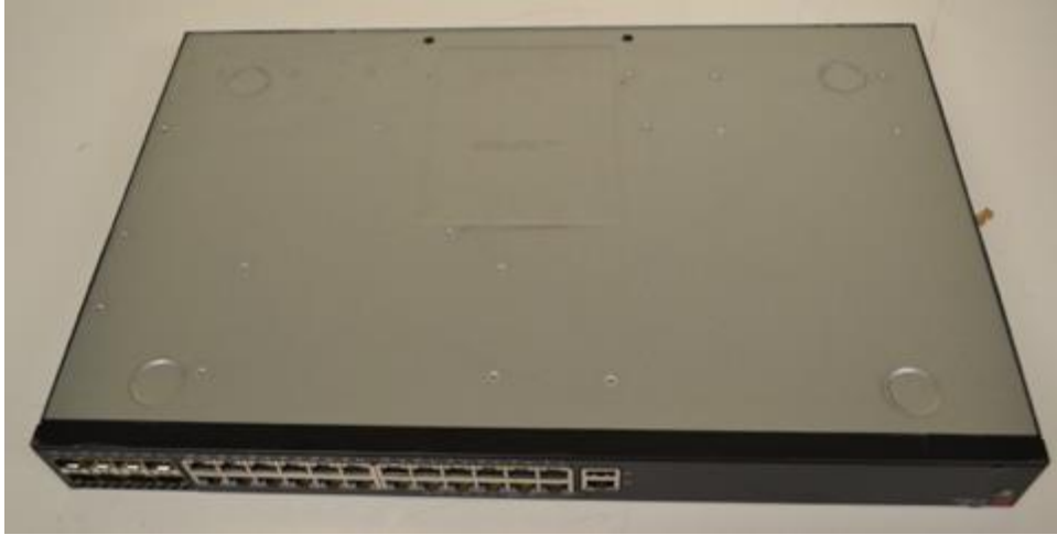
Figure 40 - Bottom side of the module ICX7250-24
