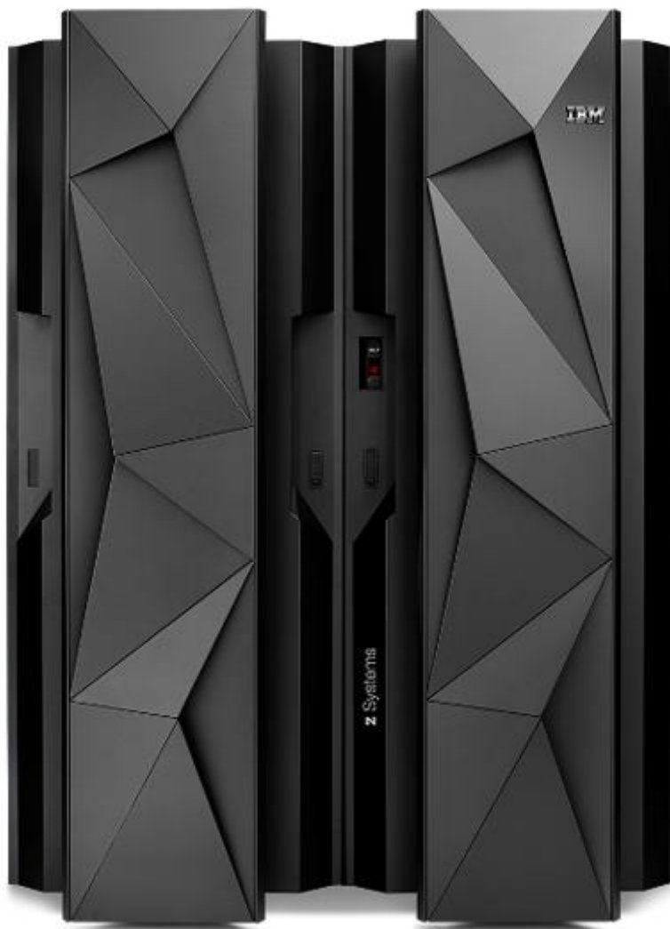
Figure 4 IBM System z13 Mainframe Computer.
