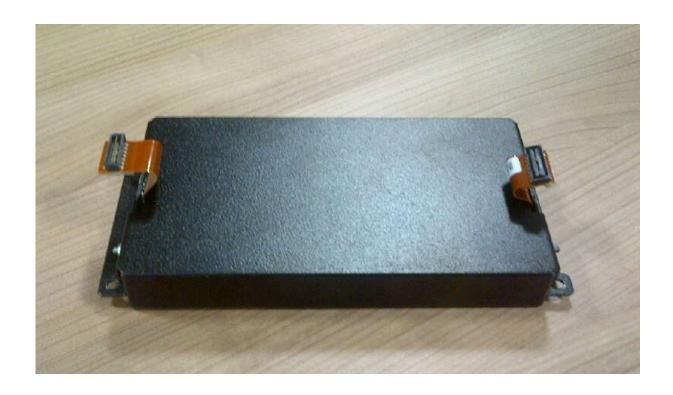
Ultra Electronics AEP's Advanced Configurable Cryptographic Environment (ACCE) v3 HSM Crypto Module
