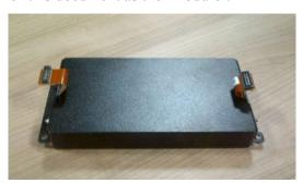
Like its predecessors, the ACCE, ACCE-L3 and ACCE v2 modules, the ACCE v3 exists to provide cryptographic services to applications running on behalf of its user which communicate with it via a standard Ethernet interface using IP protocols. To implement these services, the module additionally requires a suitable power supply, Smart Card reader, USB port, digital display device, keypad and line drivers.
