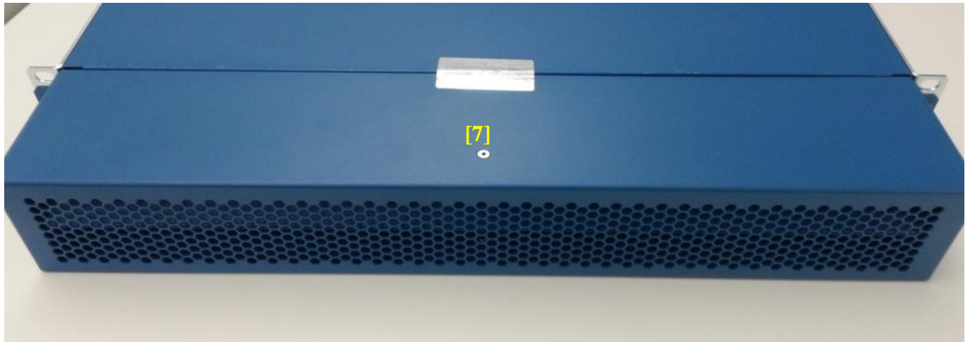
Figure 11 – PA-3060 Front/Top Tamper Seal Placement
