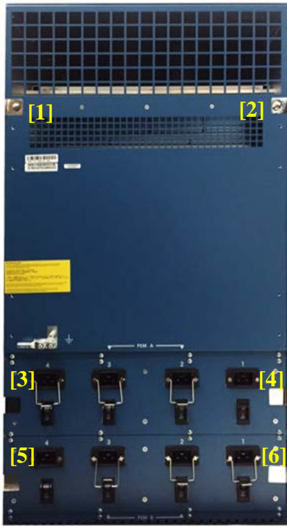
Figure 13 - PA-7080 Tamper Seal Placement for Rear (6)
