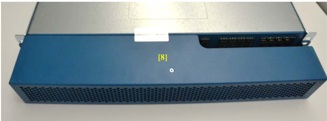
Figure 12 – PA-3060 Front/Bottom Tamper Seal Placement
