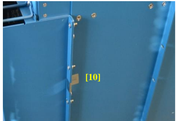
Figure 16 - PA-7080 Tamper Seal Placement on Right Side for Front Opacity Shield (1)
