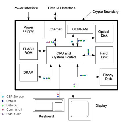
Figure 2: Cryptographic Module Physical Boundary
