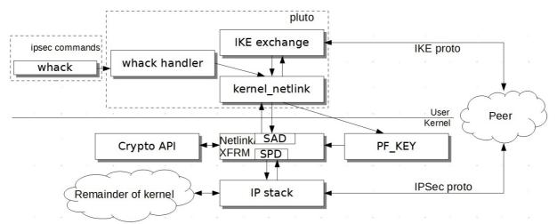
Figure 3: Relationship between Libreswan bound module and Kernel Crypto API module
