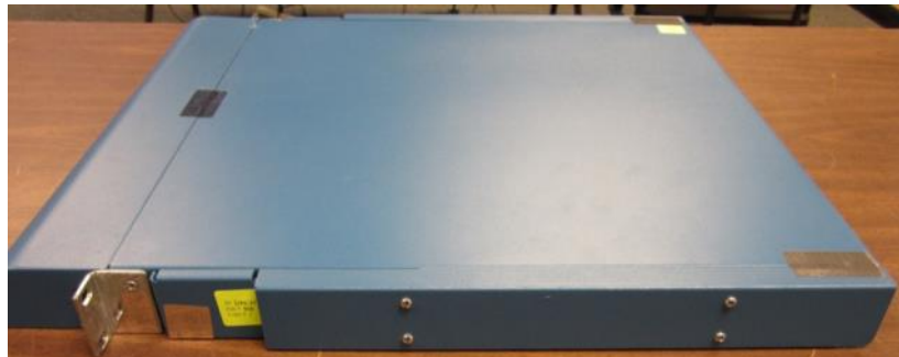
Figure 15 - PA-3020 / PA-3050 side with Opacity Shield
