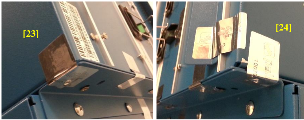
Figure 54 - PA-7050 Tamper Seal Placement for Bottom Plenum Bracket (23-24)
