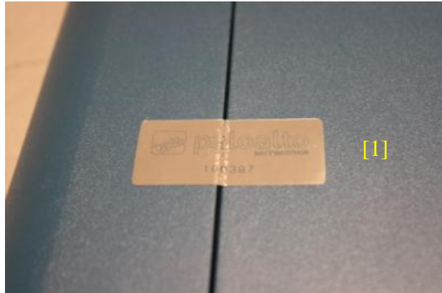
Figure 32 - PA-500 Front Tamper Seal Placement (1)
