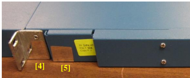
Figure 41 - PA-3020/PA-3050 Series Tamper Seal Placement (2)
