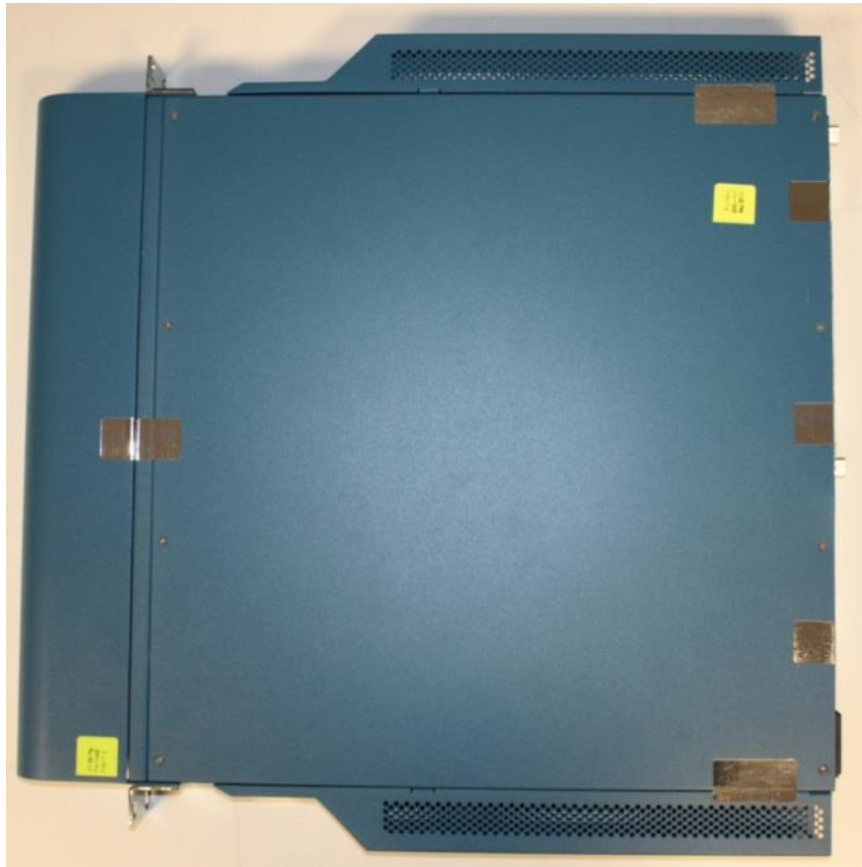
Figure 10 - PA-2020 / PA-2050 Front Opacity Shield
