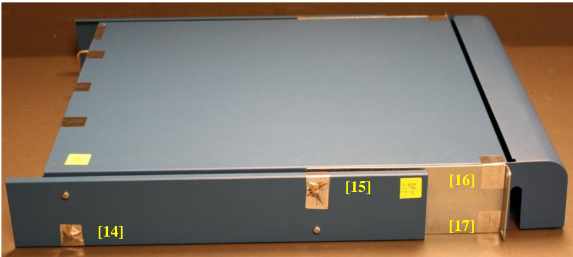
Figure 49 - PA-5000 Series Left Side Tamper Seal Placement (4)
