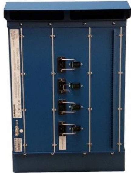
Figure 26 - PA-7050 Rear view with Opacity Shields
