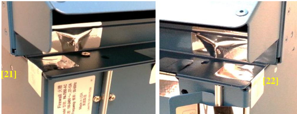
Figure 53 - PA-7050 Tamper Seal Placement for Top Plenum Bracket (21-22)
