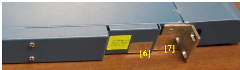
Figure 42 - PA-3020/PA-3050 Series Tamper Seal Placement (2)
