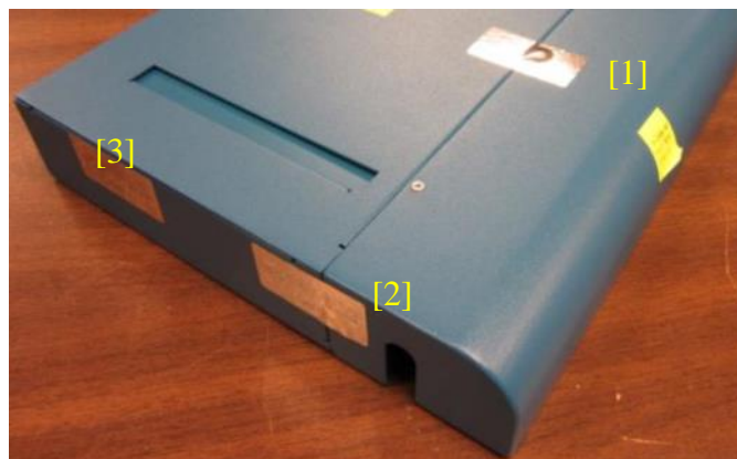
Figure 30 - PA-200 Left Side and Top Tamper Seal Placement (3)
