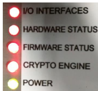
Figure 6 – Talon MFSa LED Indicator for Tamper Response
