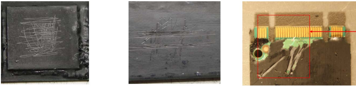
Figure 8 – MICRON 1100 M.2 Tamper Evidence
