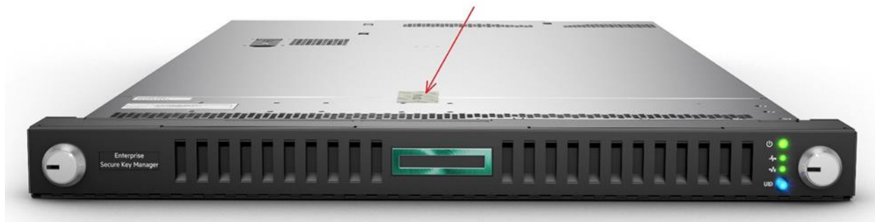
Figure 8 – Tamper-Evidence Label on ESKM
