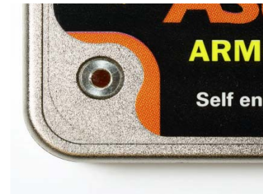
Figure 7: After Strong UV Exposure
