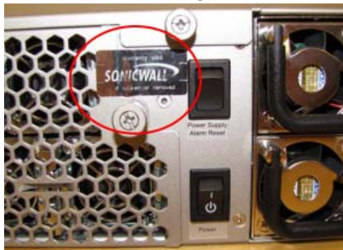
Figure 7 – SRA EX9000 Tamper Seal #5 - Rear Fans
