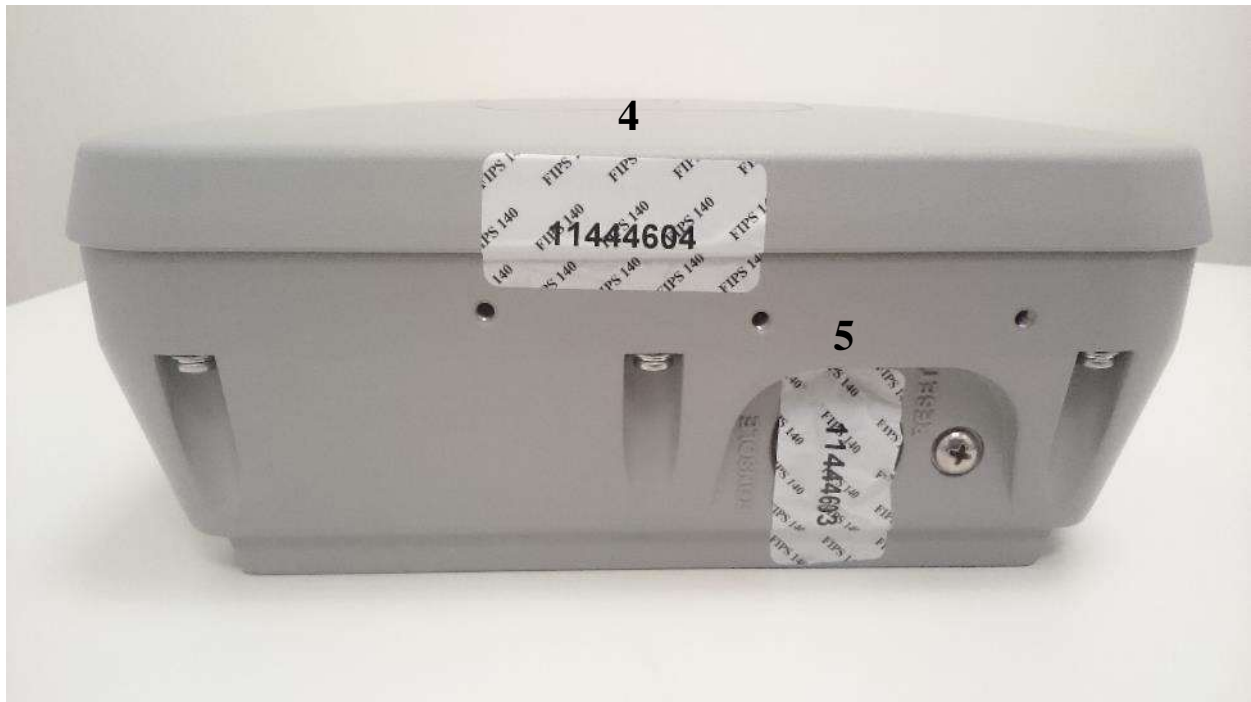
Cisco Aironet 1562i tamper label placement (Front, Back, Left, Right)
