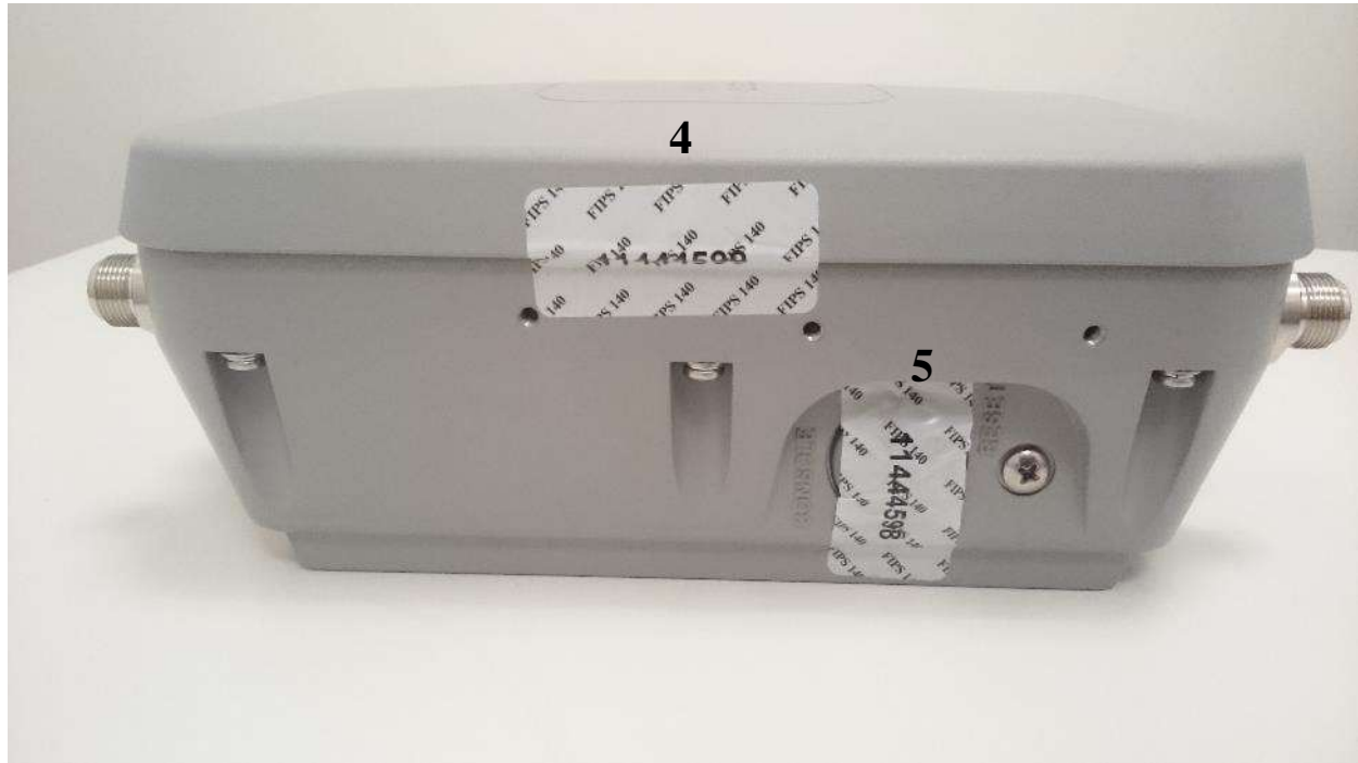
Cisco Aironet 1562e/d/ps tamper label placement (Front, Back, Left, Right)
