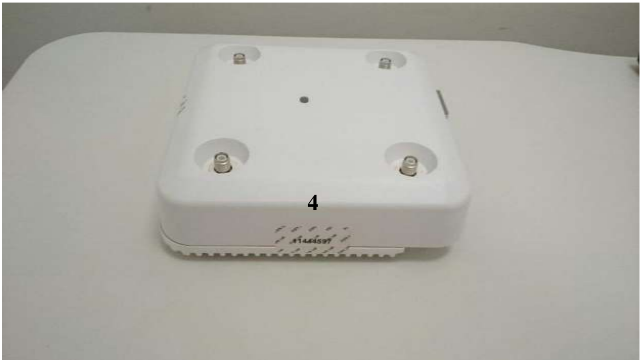
Cisco Aironet 2802e and 3802e tamper label placement (Front, Back, Left, Right)
