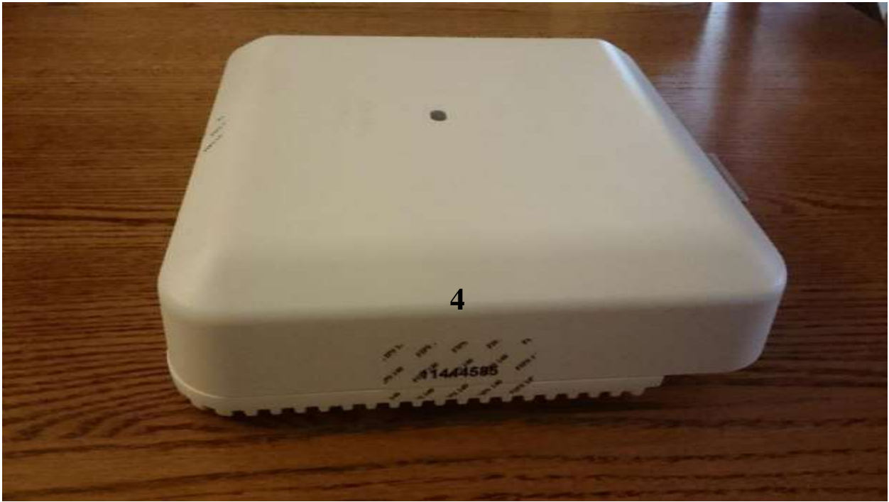
Cisco Aironet 2802i and 3802i tamper label placement (Front, Back, Left, Right)
