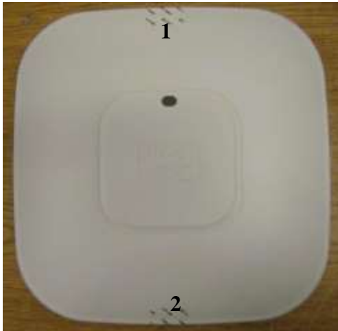
Cisco Aironet 2602e Tamper Evident Label Placement (Top, Bottom, Front, Back, Left, Right)
