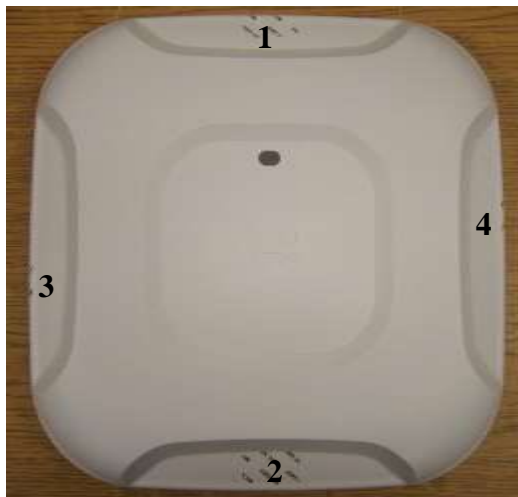
Cisco Aironet 3702e/p with AIR-RM3000M Tamper Evident Label Placement (Top, Bottom, Front, Back, Left, Right)
