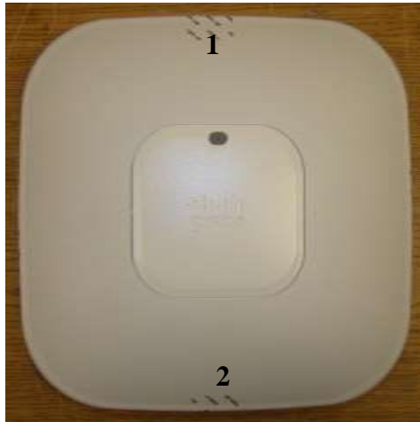
Cisco Aironet 3602e/p with AIR-RM3000M Tamper Evident Label Placement (Top, Bottom, Front, Back, Left, Right)
