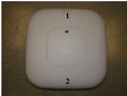
Cisco Aironet 2702e Tamper Evident Label Placement (Top, Bottom, Front, Back, Left, Right)
