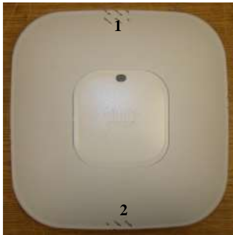
Cisco Aironet 3602e/p Tamper Evident Label Placement (Top, Bottom, Front, Back, Left, Right)
