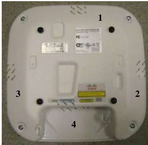
Cisco Aironet 1602e Tamper Evident Label Placement (Front, Back, Top, Bottom, Left, Right)
