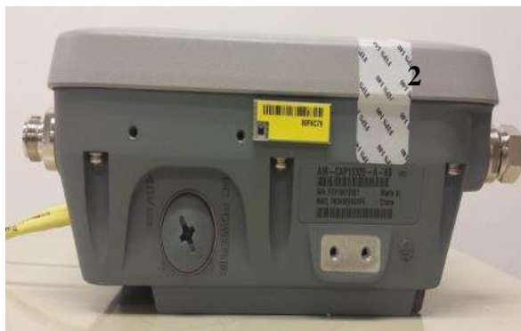
Cisco Aironet 1532e Tamper Evident Label Placement (Front, Back, Bottom, Top, Left, Right)
