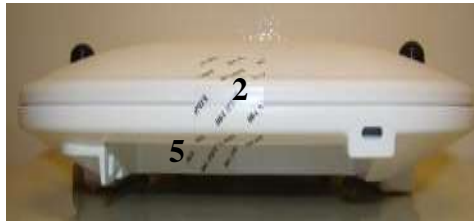
Cisco Aironet 3602e/p Tamper Evident Label Placement (Top, Bottom, Front, Back, Left, Right)
