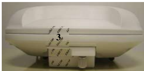
Cisco Aironet 3702i with AIR-RM3000M Tamper Evident Label Placement (Top, Bottom, Front, Back, Left, Right)
