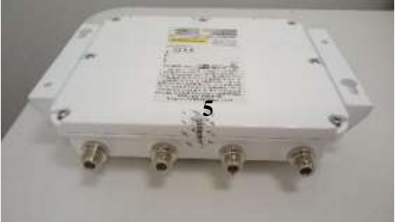
Cisco IW3702-4E Tamper Evident Label Placement (Top, Front, Back)
