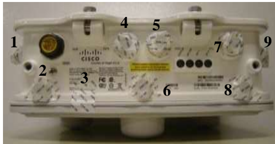
Cisco Aironet 1552e Tamper Evident Label Placement (Front, Back, Top, Bottom, Left, Right)
