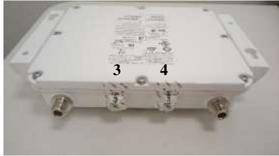
Cisco IW3702-2E Tamper Evident Label Placement (Top, Front, Back)
