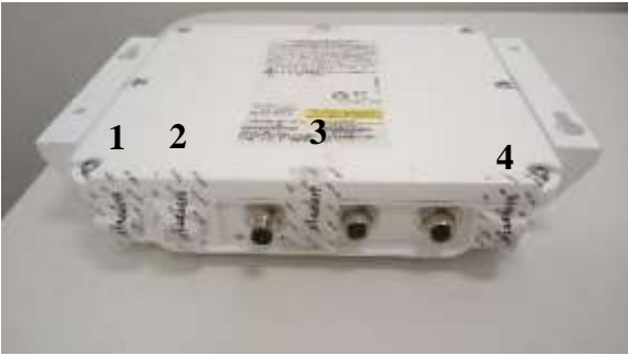
Cisco IW3702-2E Tamper Evident Label Placement (Top, Front, Back)
