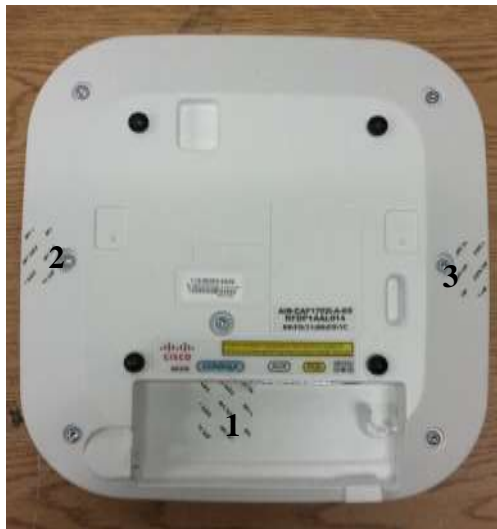
Cisco Aironet 1702i Tamper Evident Label Placement (Front, Back, Top, Bottom, Left, Right)
