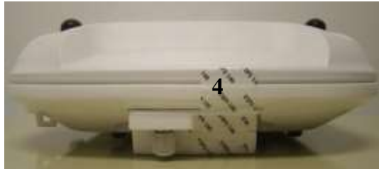
Cisco Aironet 3702e/p with AIR-RM3000M Tamper Evident Label Placement (Top, Bottom, Front, Back, Left, Right)
