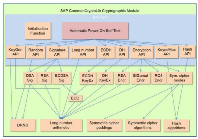
Figure 1: Block diagram of the cryptographic module
