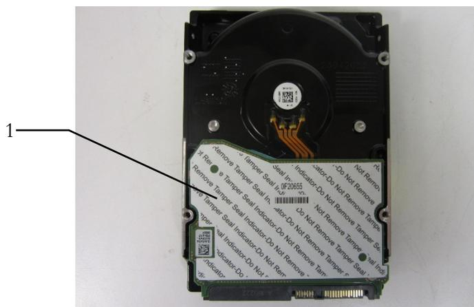
Figure 5: Tamper-Evident Seal
