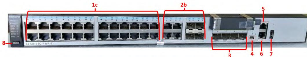
Figure 3-7: S5720-36C-PWR-EI-AC Ports – Front Panel
