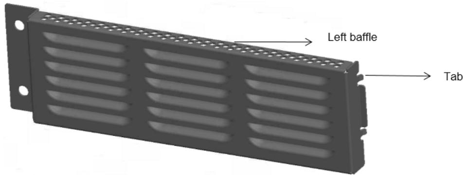
**Figure 7-2:** Insert the two tabs on the baffle into air vents on the left side of the switch.
