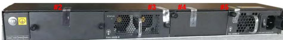
Figure 7-26: Tamper Seal Locations - Back
