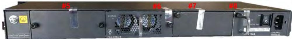
Figure 7-14: Tamper Seal Locations - Back
