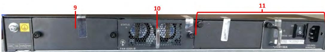
Figure 3-4: S5720-36C-EI-AC Ports – Back Panel
