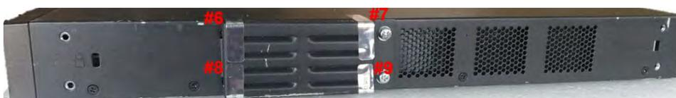
Figure 7-27: Tamper Seal Locations - Right Side Baffle
