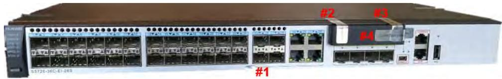
Figure 7-9: Tamper Seal Locations - Front
