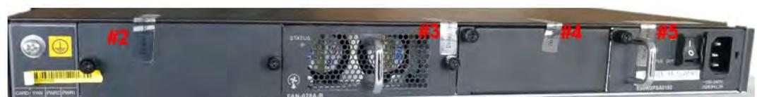
Figure 7-18: Tamper Seal Locations - Back
