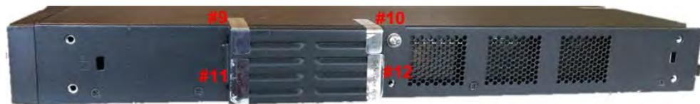
Figure 7-11: Tamper Seal Locations - Right Side Baffle
