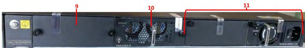
Figure 3-8: S5720-36C-PWR-EI-AC Ports – Back Panel
