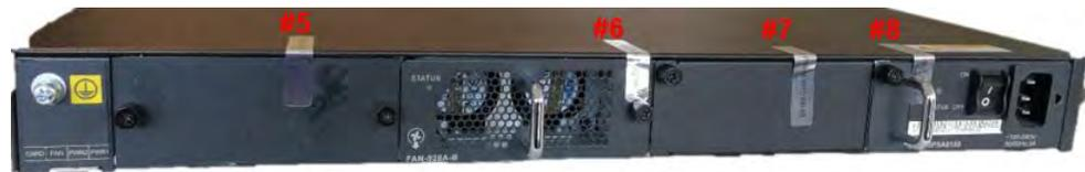
Figure 7-10: Tamper Seal Locations - Back
