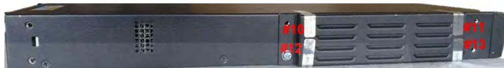
Figure 7-20: Tamper Seal Locations - Left Side Baffle
