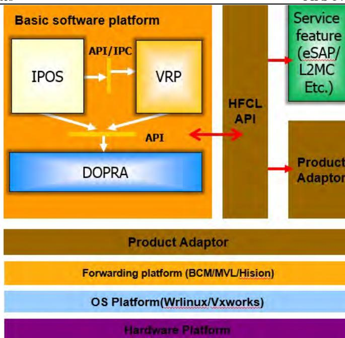
Figure 2-11: Firmware Block Diagram
