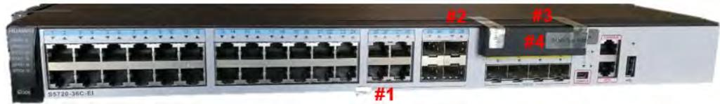
Figure 7-13: Tamper Seal Locations - Front
