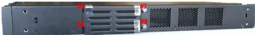
Figure 7-19: Tamper Seal Locations - Right Side Baffle
