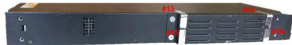
Figure 7-12: Tamper Seal Locations - Left Side Baffle
