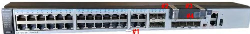
Figure 7-21: Tamper Seal Locations - Front
