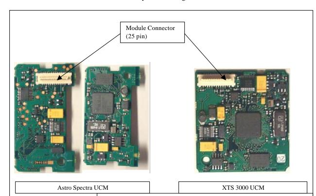
The UCM Module Connector contains all interface connections to the UCM: SPI (Data, Control, Status, OTAR Key data), SCI (Data, Control, Status), KVL (Key Data, Control, Status), and Unswitched and Switched Power Connections. It is also used for tamper detection: If the module is ever disconnected from its host Radio, a tamper will be detected and all security related data items (CSPs) will be erased.
