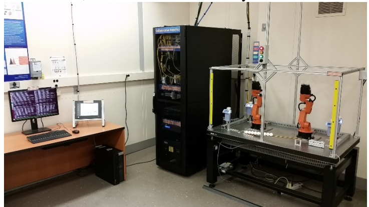
Figure 8: Collaborative robotics portion of the ICS cybersecurity testbed
