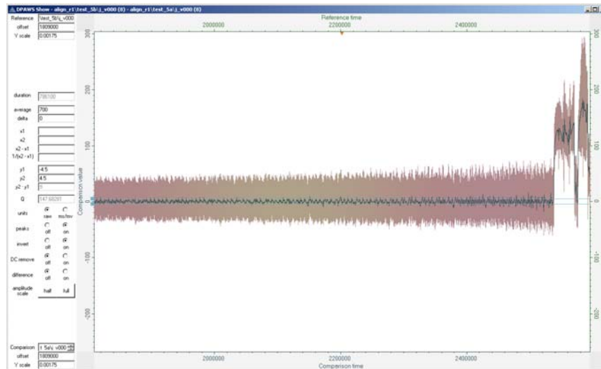
Figure 3: t-test results for Test 5 for DEVICE 1, aligned at the end of the RSA-CRT operation.
