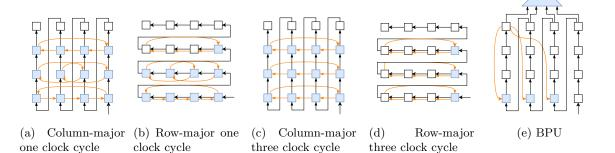
Fig. 2: ShiftRow implementations. Registers are indicated by square boxes. Black arrows indicate regular shifting operation while orange arrows indicate ShiftRows shifting. Blue registers need to be prefaced with a mux.
