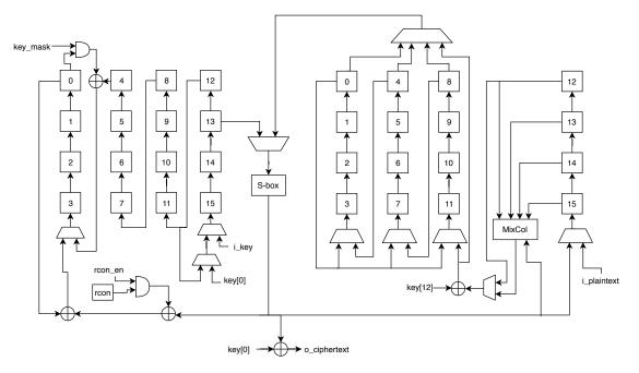
Fig. 4: Quark-AESarchitecture with key register on the left and state register on the right
