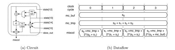
Fig. 5: Quark-AES MixColumns circuit and operation
