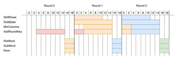
Fig. 6: Dataflow of Quark-AES showing first 3 rounds. Blocks of the same colour represent operations belonging to the same AES round.
