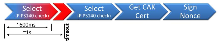
Insufficient power in card to complete the fips140 start-up checks
