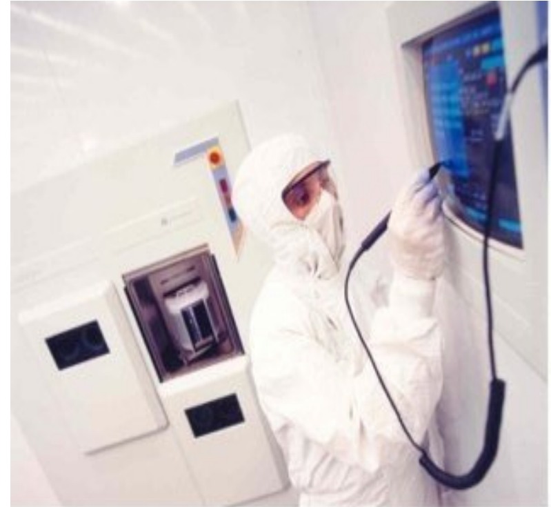
A technician programs a product "Recipe" into an epi reactor.
