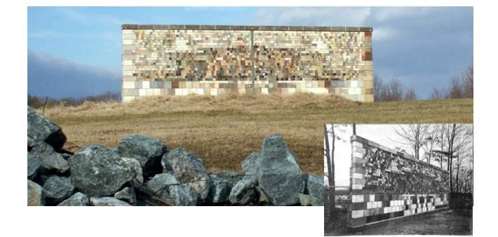
The NIST Stone Test Wall: "Constructed [in 1948] to study the performance of stone subjected to weathering. It contains 2352 individual samples of stone, of which 2032 are domestic stone from 47 states, and 320 are stones from 16 foreign countries."
