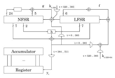
Figure 2: An overview of the initialization in Grain-128AEADv2. Note that, in hardware, the accumulator initialization is realized by first loading 64 pre-output bits into the register, followed by moving them to the accumulator.
