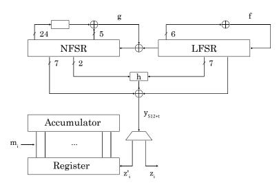
Figure 1: An overview of the building blocks in Grain-128AEADv2.
