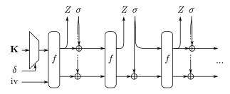
Figure 5: The full-state keyed duplex construction.
