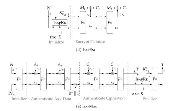
Figure 2.1.: IsaP's encryption  $\mathcal{E}(K, N, A, M)$  and decryption  $\mathcal{D}(K, N, A, C, T)$  algorithms composing IsaPENc stream encryption, IsaPMac MAC, and IsaPK re-keying.
