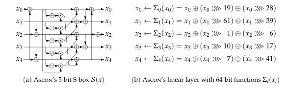
Figure B.1.: Ascon's substitution layer and linear diffusion layer.
