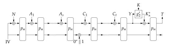
Figure 4.2.: Sketch of authentication/verification just using a sponge-based suffix MAC. Here,  $g'_2 = g_2 \oplus id$ .
