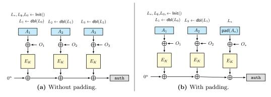
Figure 1: Processing of the associated data in OCB.
