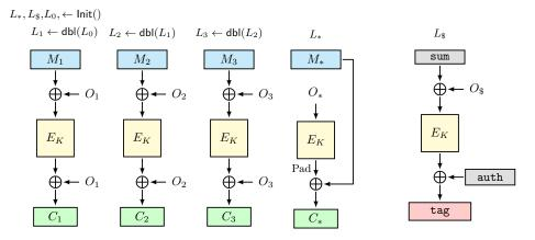
Figure 2: Encryption part of OCB.
