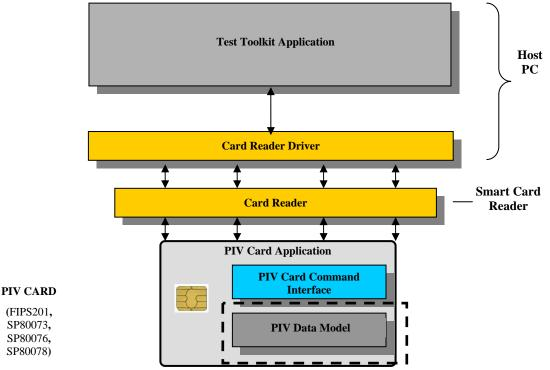
Figure 1: PIV Conformance Test Architecture
