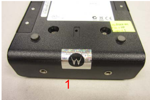
Figure 7: Tamper-Evident Seal #1 (Underside Left Side)
