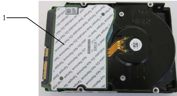
Figure 5: Tamper Evident Seal
