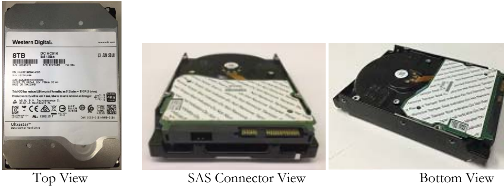
Figure 4: Ultrastar DC HC510 Cryptographic Boundary, Hardware Version 2
