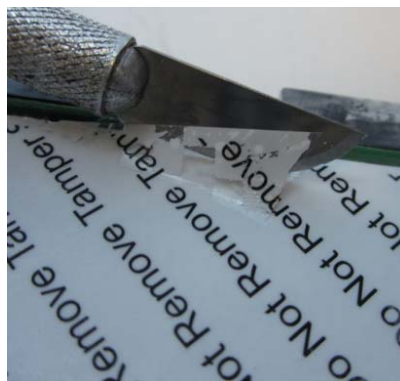
Figure 6: Tamper Evidence on Tamper Seal
