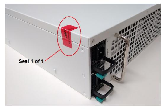
Figure 6: FortiGate-3815D Enclosure Seal, top, right side
