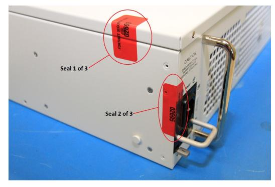
Figure 4: FortiGate-3700D Enclosure Seal and Power Supply Seals, rear, right side
