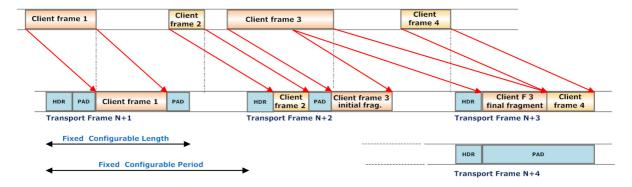
Figure 7 – TRANSEC constant rate transport frame assembly
