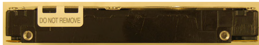
Figure 9: Right-side view of tamper-evidence label on right side of Enterprise Performance HDD v9, 2.5-Inch, 10K-RPM, SAS Interface module
