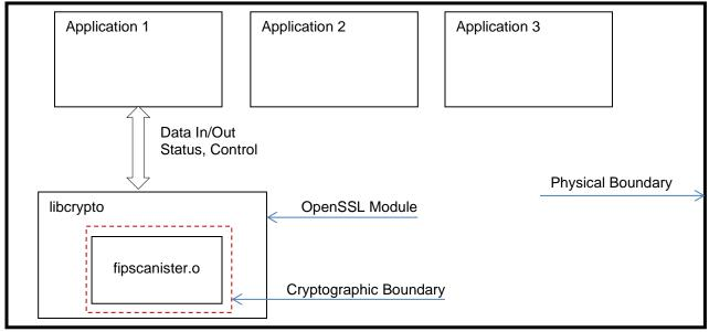
Figure 1 – Software Block Diagram
