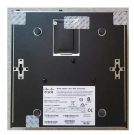
Figure 30 ASA 5506H-X Bottom TEL Placement
