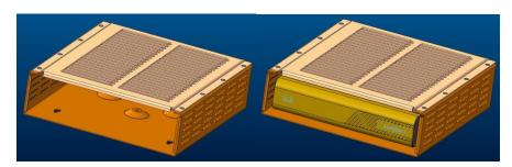
Figure 16 ASA 5506-X, ASA 5506H-X and ASA 5506W-X Opacity Shield Placement
