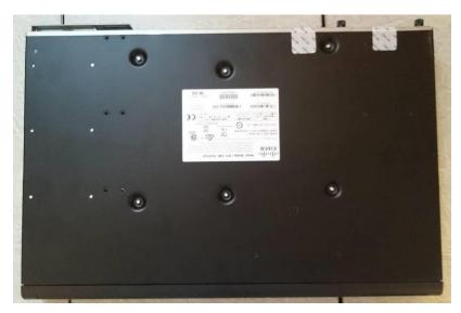
Figure 36 ASA 5508-X Bottom TEL Placement
