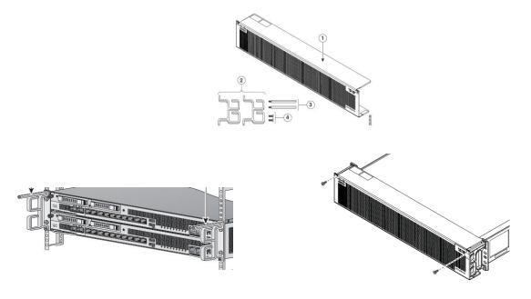
Figure 18 ASA 5585-X Opacity Shield Placement
