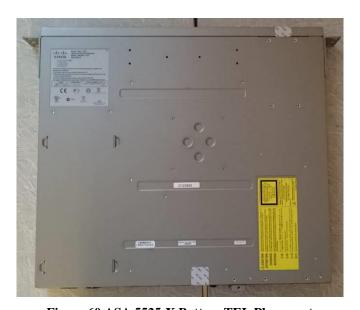
Figure 60 ASA 5525-X Bottom TEL Placement
