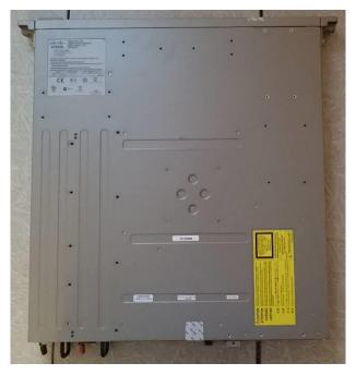
Figure 72 ASA 5555-X Bottom TEL Placement
