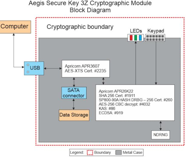
Figure 2 – Aegis Secure Key 3Z Cryptographic Module Block Diagram
