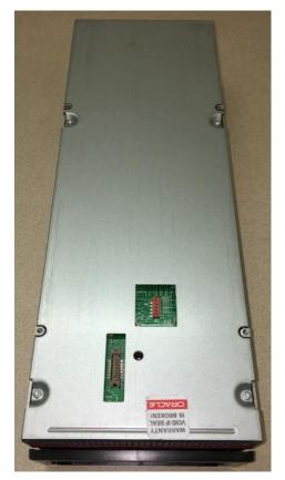
Figure 5 – StorageTek T10000D Tape Drive (Bottom)<sup>13</sup>
