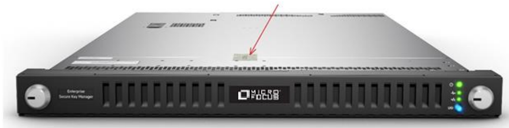
Figure 9 – Tamper-Evidence Label on ESKM
